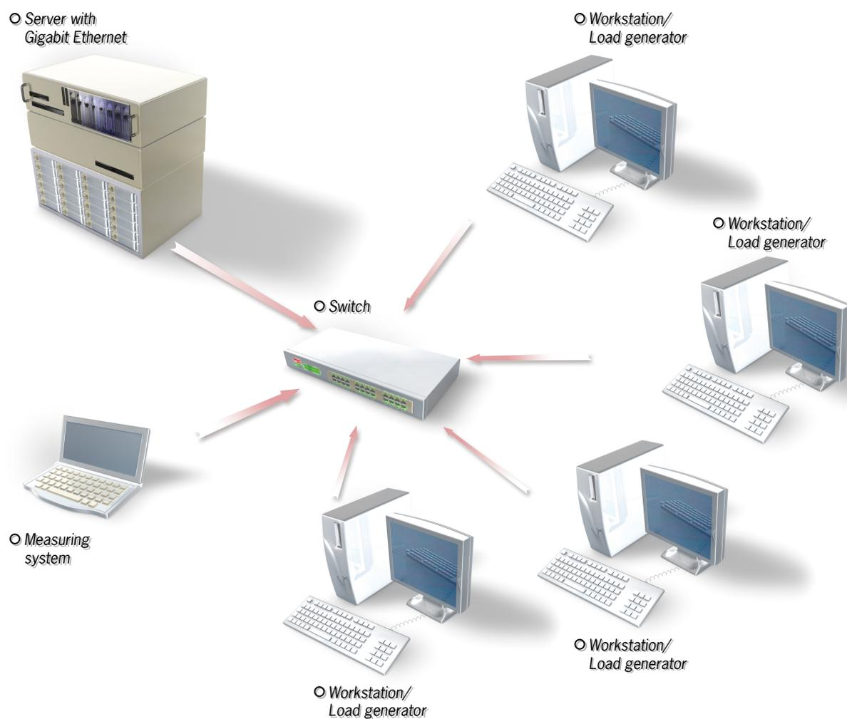
Figure 5: Test environment for variable client number
