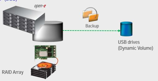
Data residing on DSS is backedup from the RAID Array to USB Drive as a (Dynamic Volume) for NAS shares.
