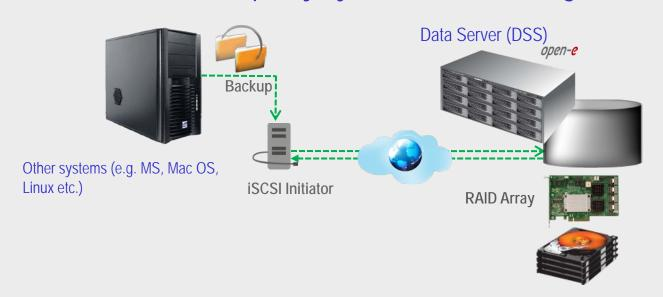
Data is backed up from the other system to a iSCSI target via the WAN on the RAID Array of the Data Server (DSS).
