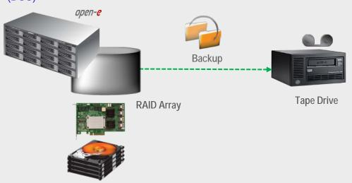
Data residing on DSS is backed up from RAID Array to Tape Drive.
