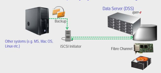
Data is backed up from the other system to FC target via the LAN on the RAID Array of the Data Server (DSS).
