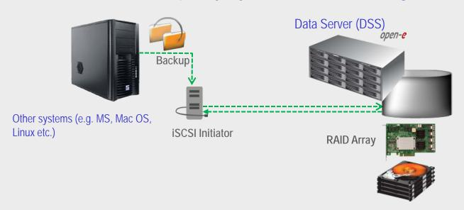
Data is backed up from the other system to the iSCSI target via the LAN on the RAID Array of the Data Server (DSS).
