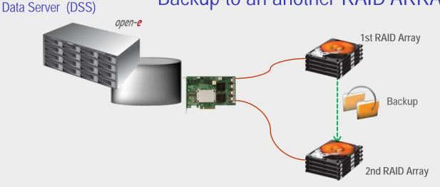
Data residing on DSS is backedup from 1st RAID Array to 2nd RAID Array using the built-in Local Backup functions for NAS shares.
