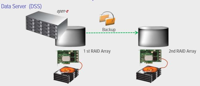
Data residing on the DSS is backed up from 1st RAID Array to 2nd RAID Array using built-in Local Backup functions for NAS shares.
