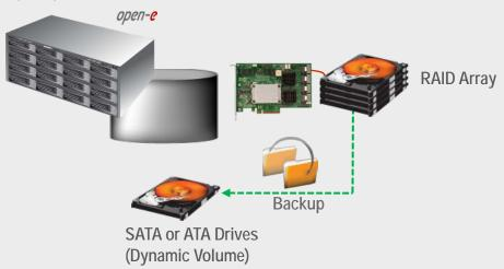
Data residing on DSS is backedup from the RAID Array to ATA or SATA Drives as a Dynamic Volume for NAS shares.
