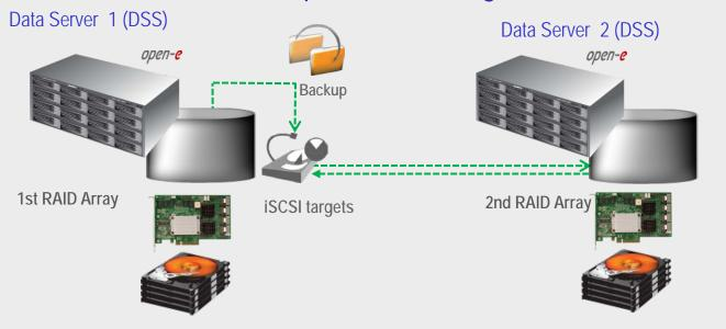
Data residing on DSS 1 is backedup from 1st RAID Array to the iSCSI target, available via the LAN on the DSS 2 using built-in Local Backup functions for the NAS share.
