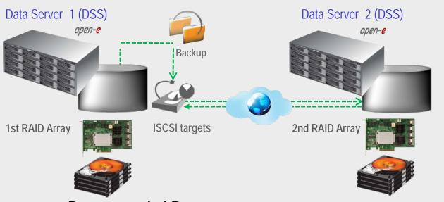
Data residing on DSS1 is backed up from 1st RAID Array to iSCSI target volume available via the WAN on the DSS 2 using built-in Local Backup functions for the NAS share.
