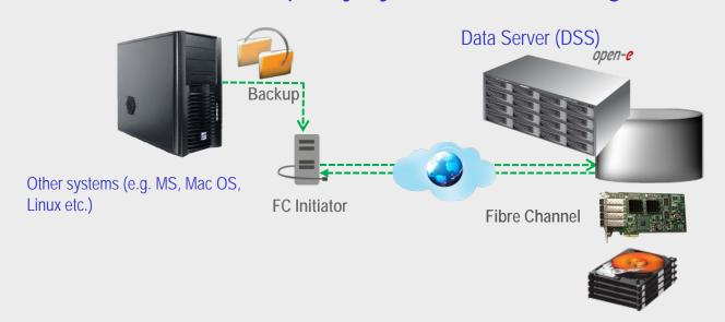
Data is backed up from the other system to the FC target via WAN on the Fibre Channel of the Data Server (DSS).
