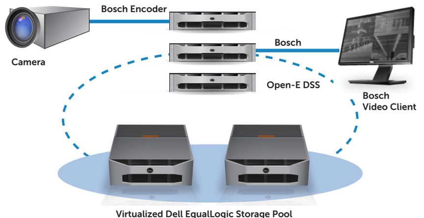
Dell EqualLogic unified, virtualized IP storage, Open-E Data Storage Software and Bosch Video Management System enables affordable video management with simplified management and high scalability.
