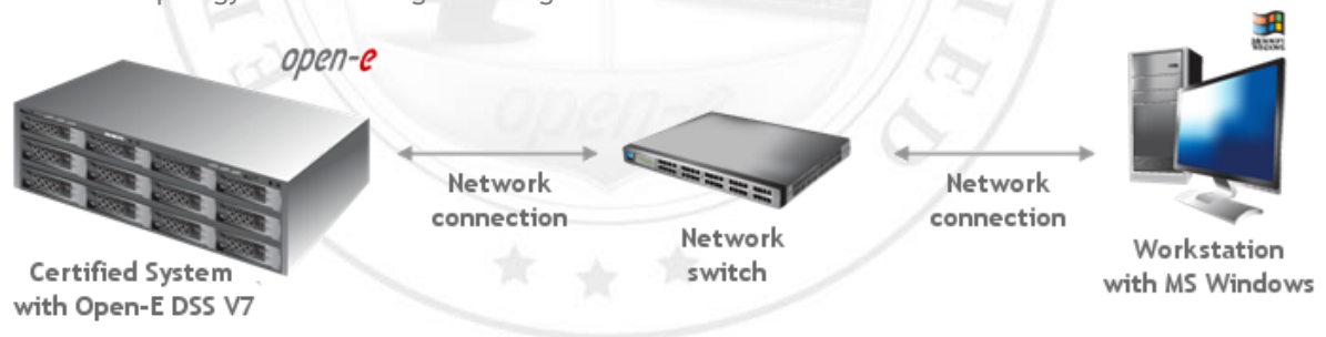
FIGURE 26: Network topology for iSCSI Target testing
