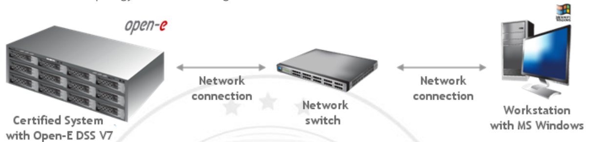
FIGURE 16: Network test topology for RAID testing
