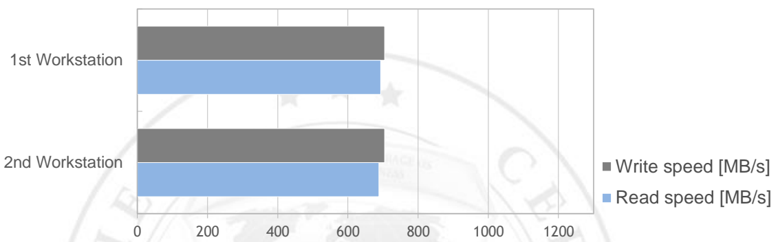
FIGURE 9: Balance-alb bonding mode performance test results chart for Intel® Ethernet Converged Network Adapter X540-T2
