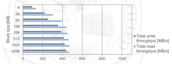
FIGURE 2: Active-Passive iSCSI Failover data throughput performance test results chart for Broadcom 5720 Quad-Port 1GbE on one active node
