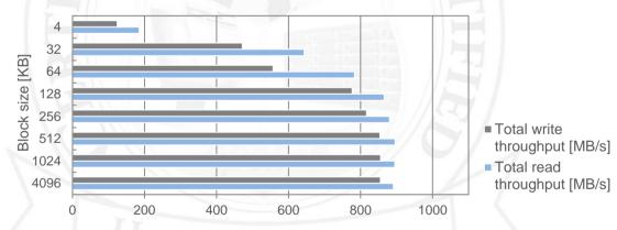
FIGURE 3: Active-Active iSCSI Failover data throughput performance test results chart for Broadcom 5720 Quad-Port 1GbE on both active nodes
