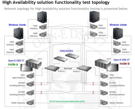
FIGURE 6: Network topology for High Availability solution functionality testing
