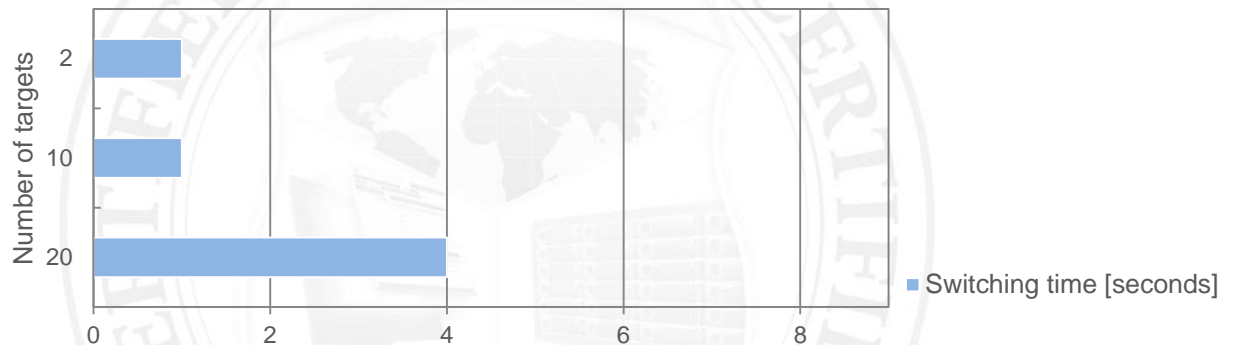
FIGURE 4: Active-Passive iSCSI Failover resource group switching time test chart for QLogic QLE3442-CU on one active node
