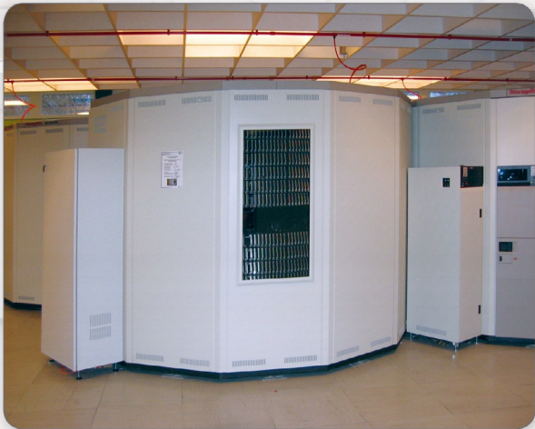
The raw data store - the tape library - is DESY's data treasure chamber. Despite the use of robotics, a tape storage system is far too slow for DESY's requirements, which is why the data has to be made available on file servers.
