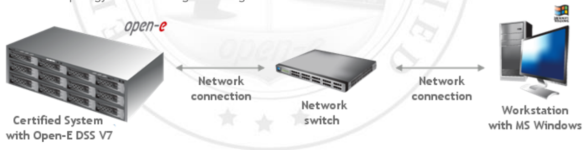
FIGURE 17: Network topology for iSCSI Target testing
