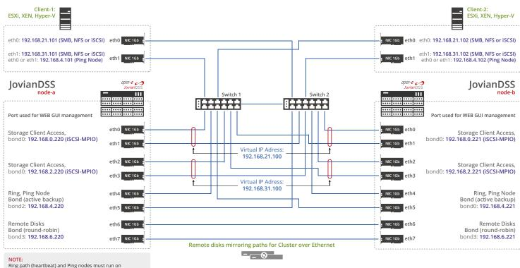
Ring path (heartbeat) and Ping nodes must run on Active-Backup bonding. Ring and Ping IP must be configured in the same network subnet.
