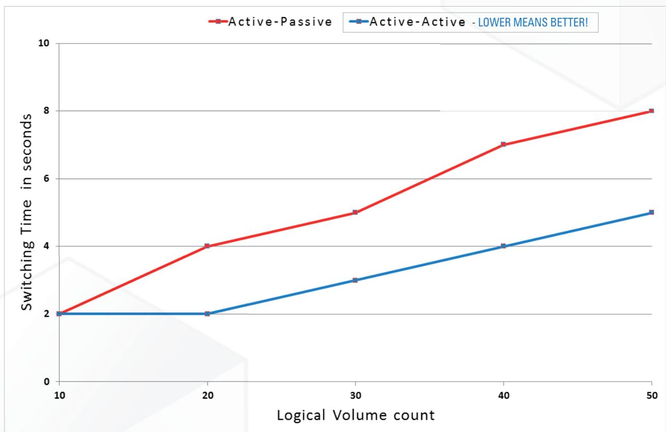
Figure 3. Failover switching time in seconds per LV count.
