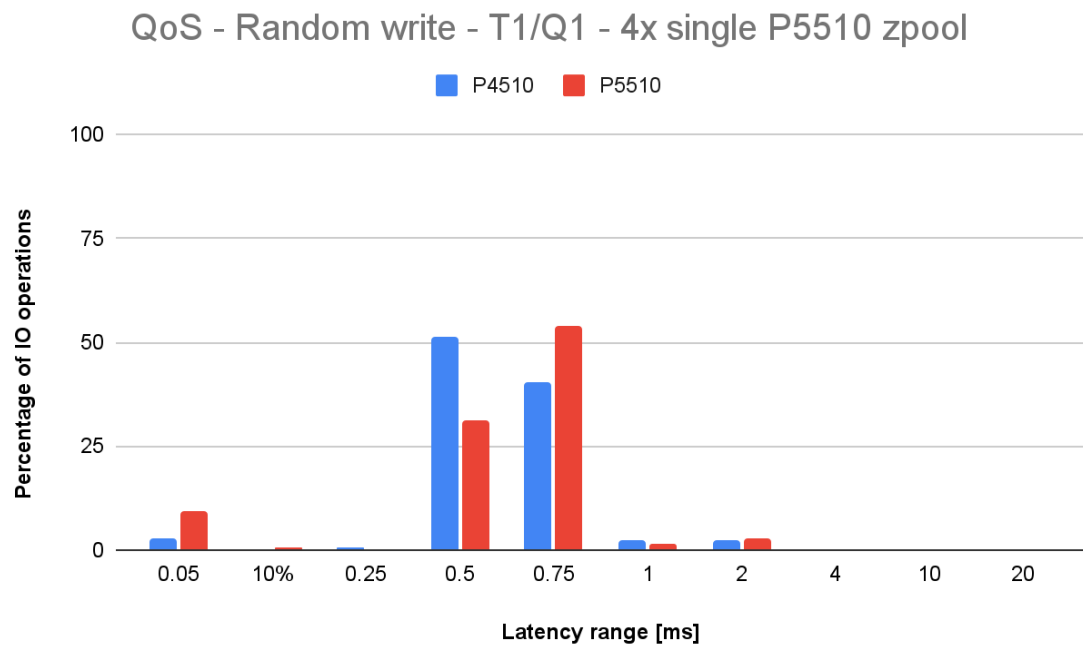
Fig. 9. Latency distribution for a random write test, done on a 4x single-disk data group zpool (T1/Q1).
