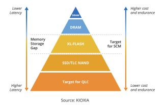
Volatile memory solutions such as DRAM provide the access speed required by demanding applications, but on the other hand, it comes at a high cost. The KIOXIA FL6 NVMe™ SSDs address this by providing high density, lower cost, and non-volatile flash memory.
