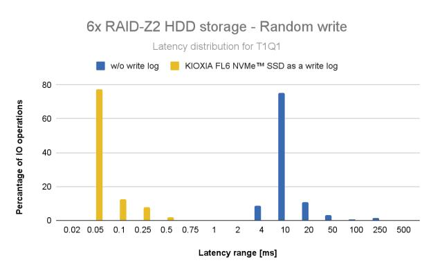
Fig. 20 Random write latency distribution for T1Q1 with 6x RAID-Z2 HDD storage.
