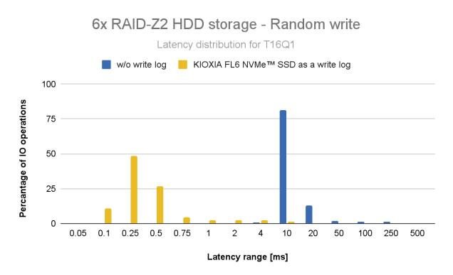
Fig. 21 Random write latency distribution for T16Q1 with 6x RAID-Z2 HDD storage.
