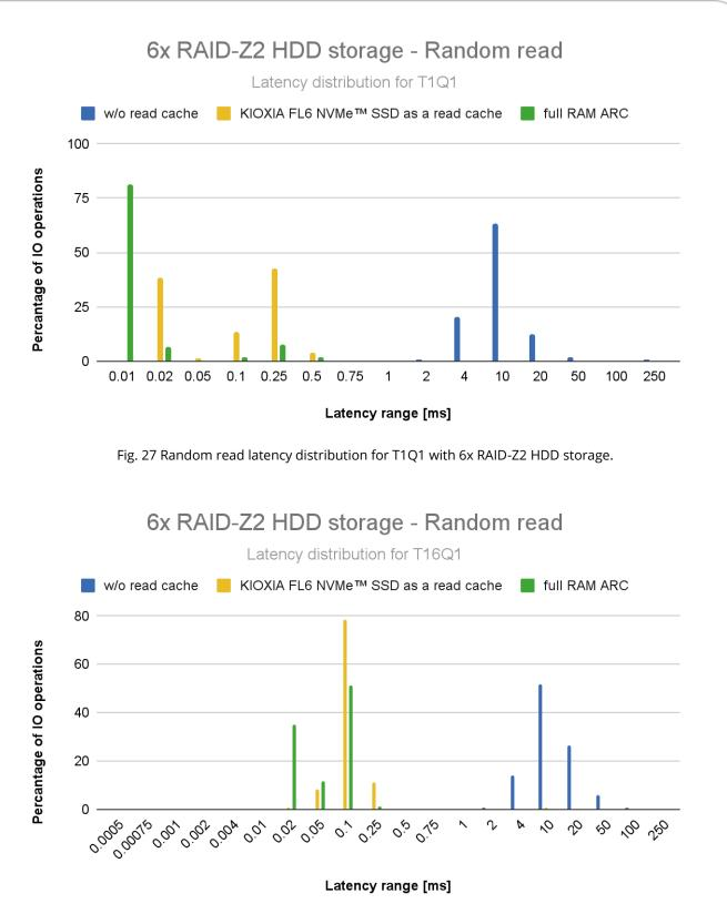
Fig. 28 Random read latency distribution for T16Q1 with 6x RAID-Z2 HDD storage.
