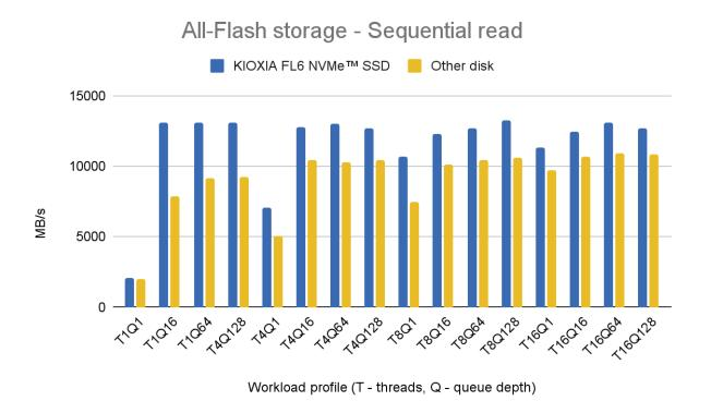
Fig. 12 Sequential read performance on the All-Flash storage, compared to a similar device.
