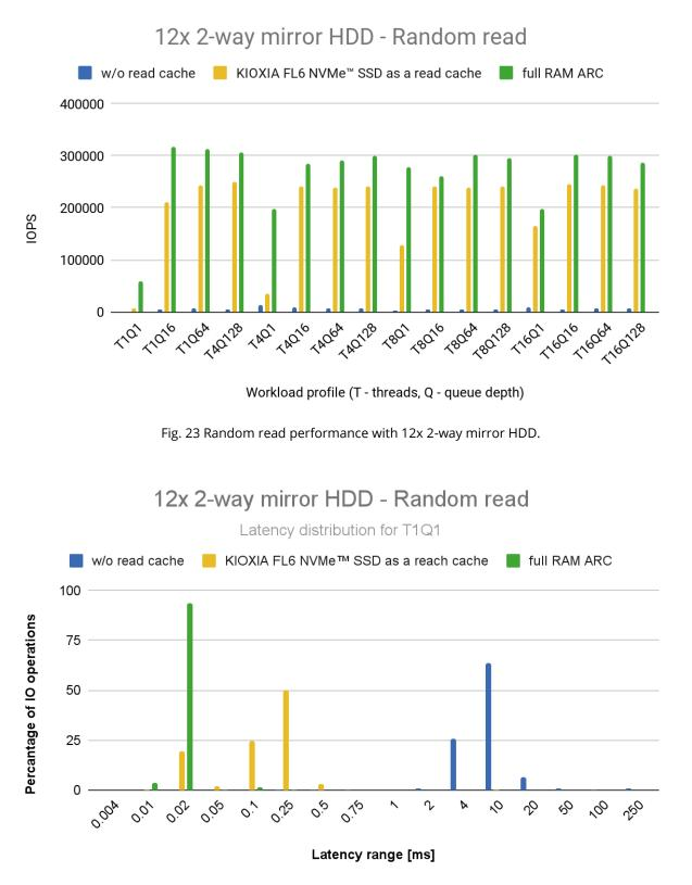
Fig. 24 Random read latency with 12x 2-way mirror HDD.
