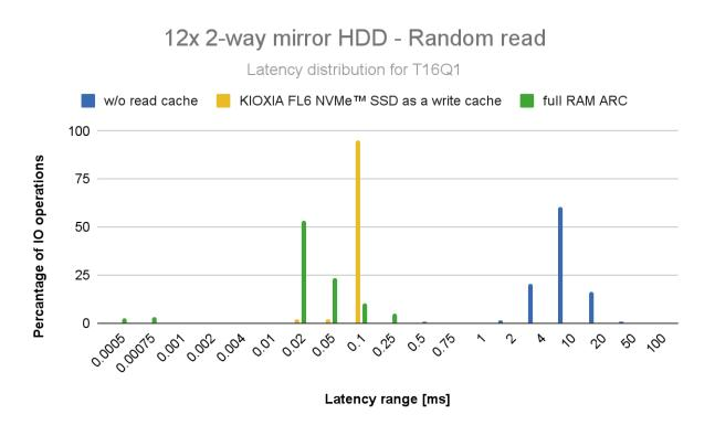
Fig. 25 Random read latency distribution for T1Q1 with 12x 2-way mirror HDD.
