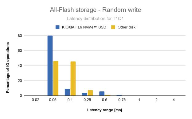
Fig. 10 Random write latency distribution for T1Q1 on the All-Flash storage, compared to a similar device.
