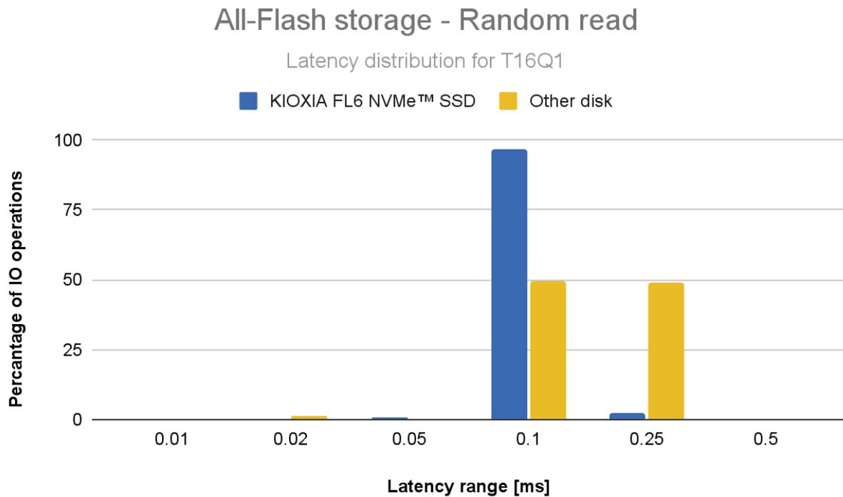
Fig. 8 Random read latency distribution for T16Q1 on the All-Flash storage, compared to a similar device.
