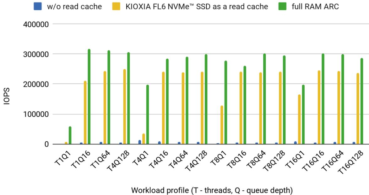
Fig. 23 Random read performance with 12x 2-way mirror HDD.
