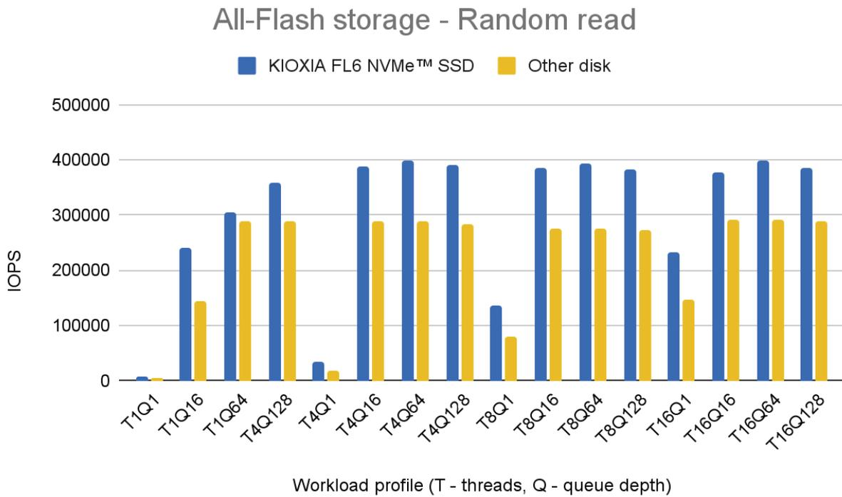
Fig. 6 Random read performance of the All-Flash storage, compared to a similar device.
