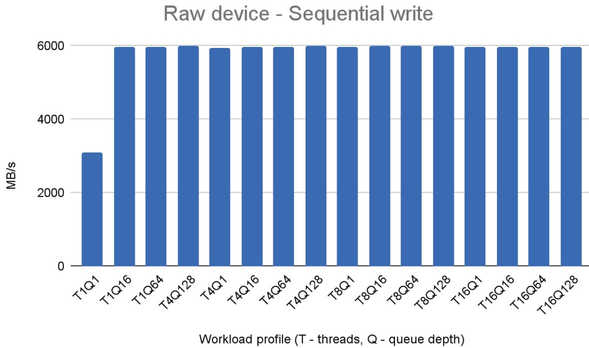
Fig. 4. Sequential write performance on the raw device.
