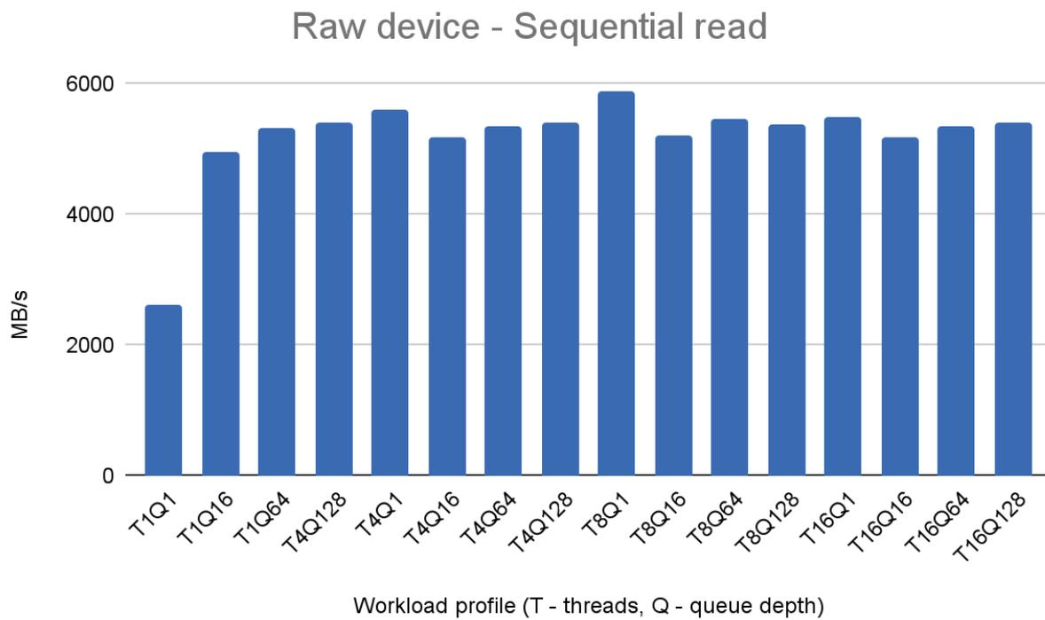
Fig. 3. Sequential read performance on the raw device.
