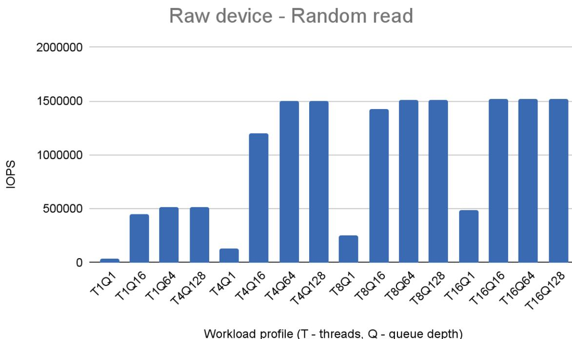
Fig. 1. Random read performance on the raw device.
