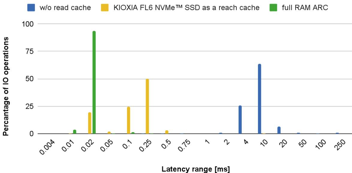
Fig. 24 Random read latency with 12x 2-way mirror HDD.
