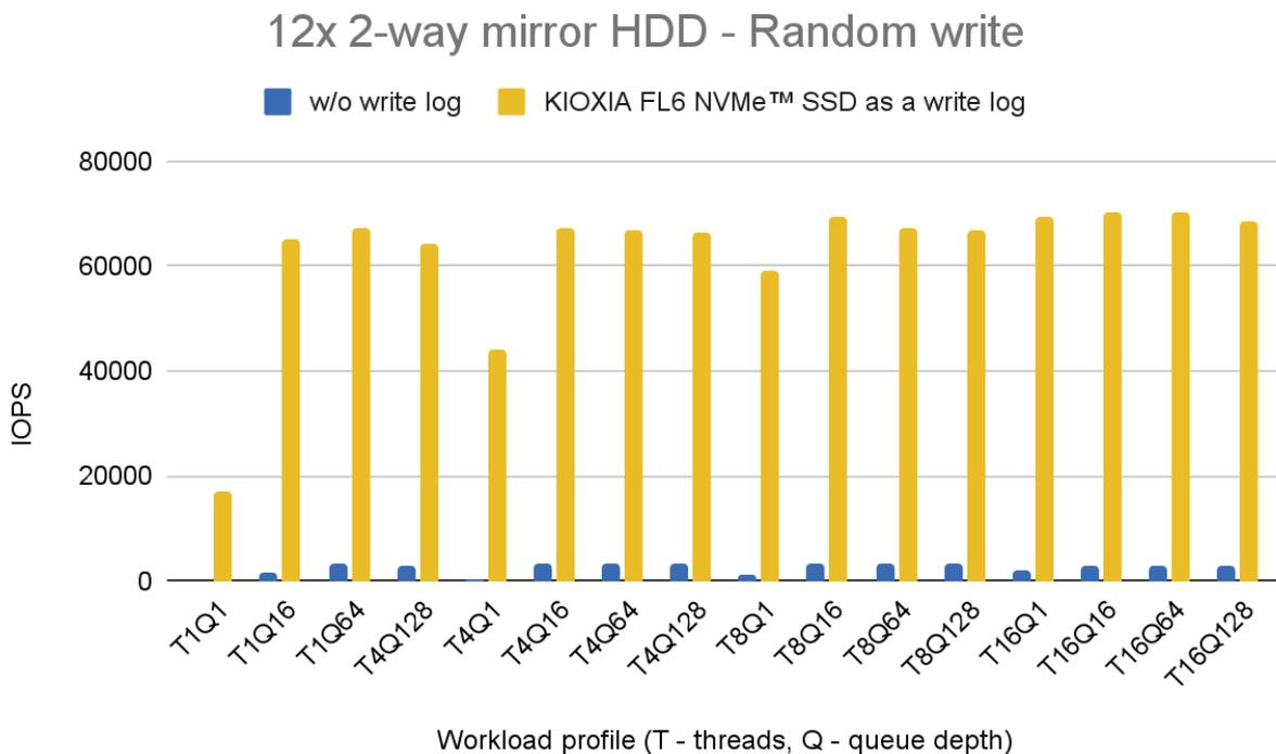
Fig. 15 Random write performance with 12x 2-way mirror HDD.
