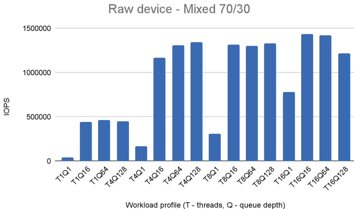
Fig. 5. Mixed 70/30 performance on the raw device.
