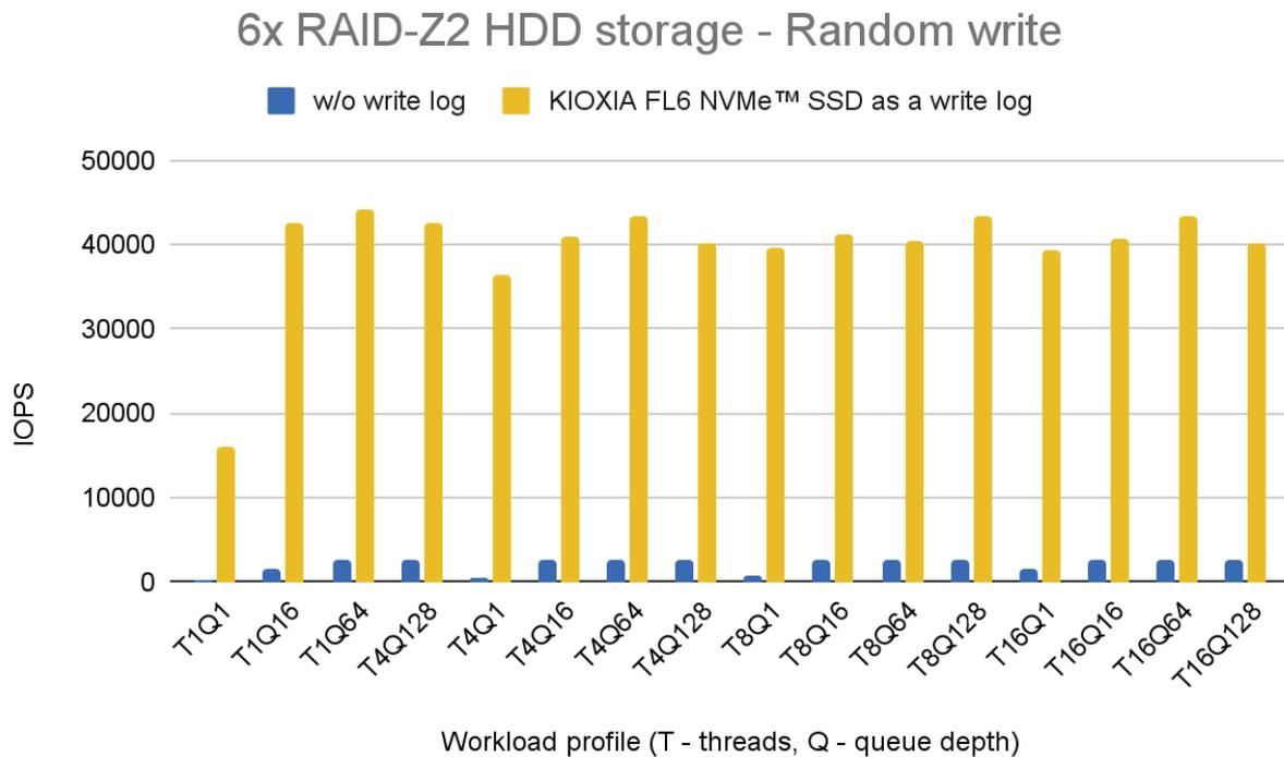
Fig. 19 Random write performance with 6x RAID-Z2 HDD storage.
