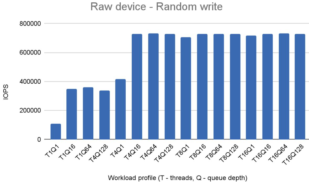
Fig. 2. Random write performance on the raw device.
