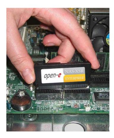
In the package you will find an adapter cable which provides Open-E NAS-XSR with power. The little white plug corresponds with the matching connector on Open-E NAS-XSR. As a final step, the adapter has to be connected to the white power-supply plug (see photo):
