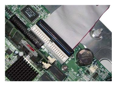
Every motherboard has at least two such ports. To install Open-E NAS-XSR, you have to use the first (primary) port.
