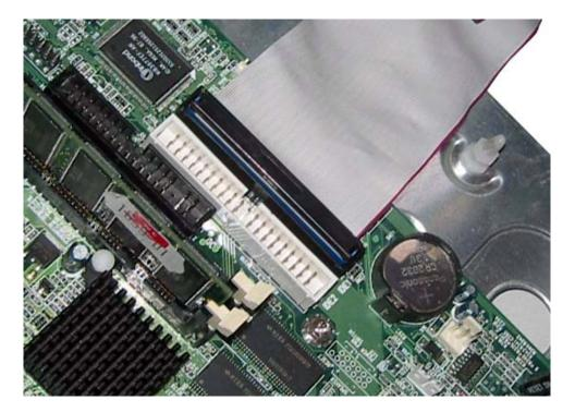
Every motherboard has at least two such ports. To install Open-E NAS-XSR, you have to use the first (primary) port.
