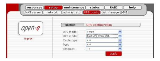
In the UPS Configuration function you can select a UPS device desired (Uninterrupted Power Supply). For the connection of the UPS device to the NAS server, the USB port is most frequently used. In the settings you can select the UPS model, cable type, connection port and the length of the time out. The time-out defines the time between a power failure and the moment the system will shut down. UPS support 3 modes:
