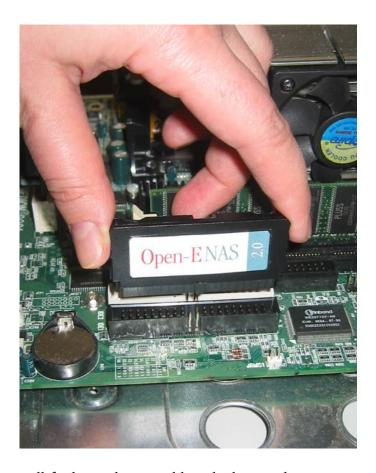
In the package, you will find an adapter cable, which provides Open-E NAS with electricity. The little white plug corresponds with the matching connector on Open-E NAS. In a final step, the adapter has to be connected to the white power-supply plug (see photo):
