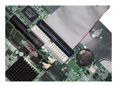
Every mainboard has at least two such ports. To install Open-E NAS, you have to use the first port because your computer "expects" this to be the position from which the booting process starts. In this example, this will soon be Open-E NAS.
