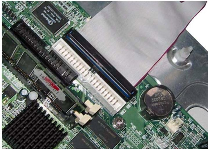
Every motherboard has at least two such ports. To install Open-E NAS, you have to use the first (primary) port.
