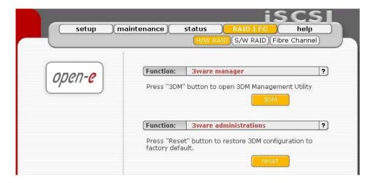
Please note that the RAID controller should be supported by the Open-E software. If a 3ware controller is installed you can click on RAID in the menu and the 3ware web base will start automatically.
