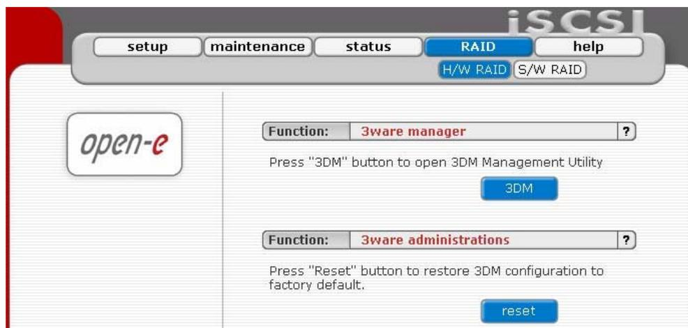
Please note that the RAID controller should be supported by the Open-E software. If a 3ware controller is installed you can click on RAID in the menu and the 3ware web base will start automatically.
