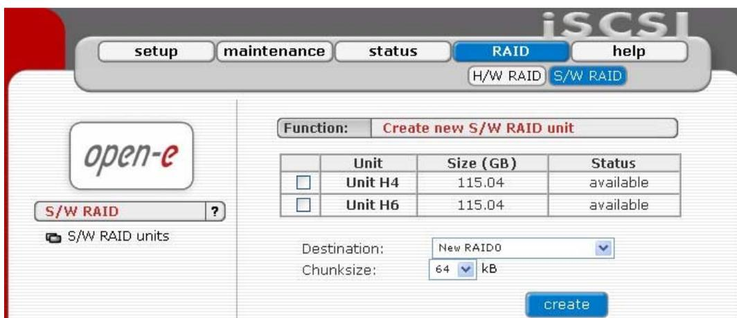
After clicking “create” button, the status will change to “in use” with additional information describing the kind of a disk array (e.g. MD0 is RAID 0)
