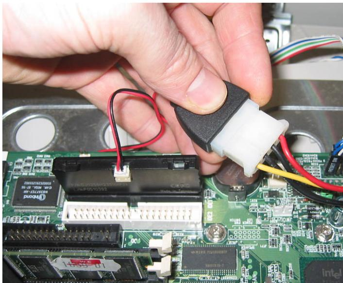
That should conclude the installation! Before putting the enclosure on your computer again, do not forget to connect your hard drives to the IDE second connector, SATA connector or to the SATA port on the RAID controller.
