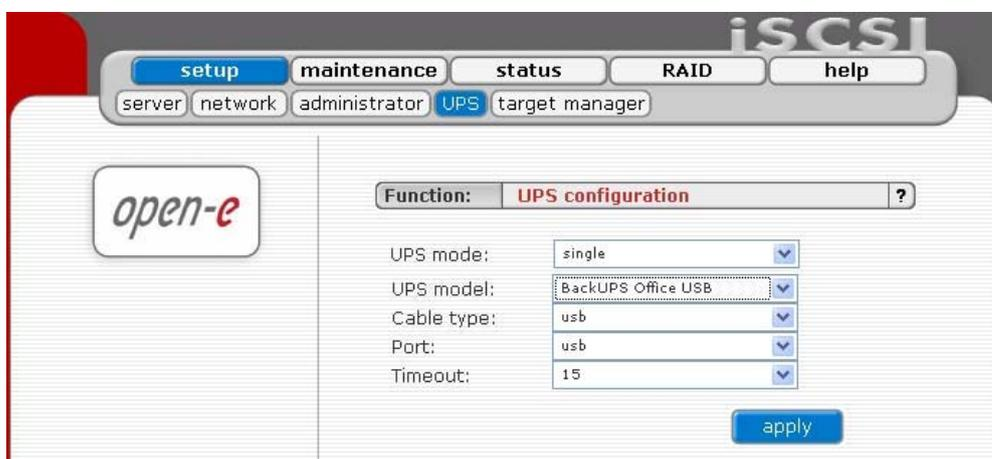
In the settings you can select the UPS model, cable type, connection port and the length of the time out. The time-out defines the time between a power failure and the moment the system will shut down. UPS support in mode “Simple” means that Open-E iSCSI is the only system attached to this UPS and that there is no action necessary to do remote shutdown for other systems in the network.
