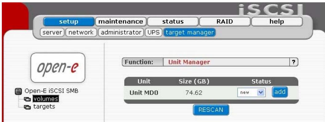
Please note that you can expand the storage capacity by adding new disk drives. In the “Unit Manager” Function Open-E iSCSI will show both 'in use' and new units. In order to add a new unit to the Volume Group (vg0), please simply click 'Add' after which Open-E iSCSI page will be restarted (see below).
