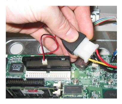
That should conclude the installation! Before putting the enclosure on your computer again, do not forget to connect your hard drives to the IDE second connector or SATA connector.
