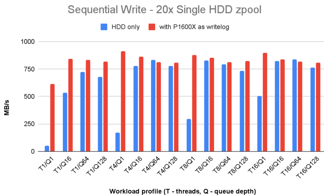
Fig. 19. Sequential write performance of a 20x single HDD zpool, with and w/o writelog.
