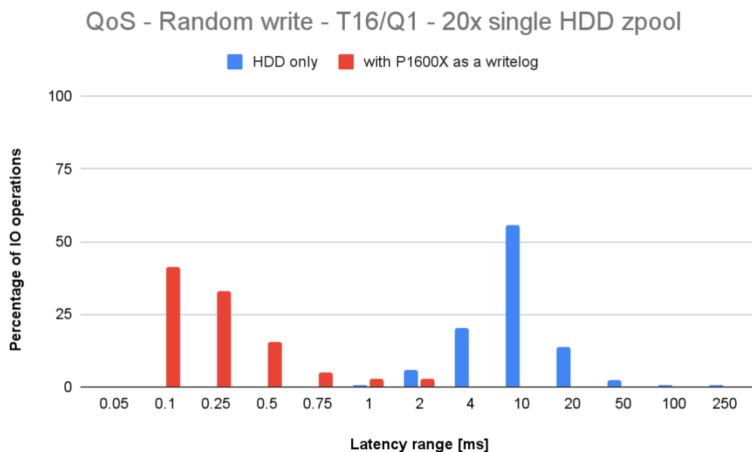
Fig. 18. Latency distribution for a random write test, done on a 20x single HDD zpool (T16/Q1), with and without writelog.
