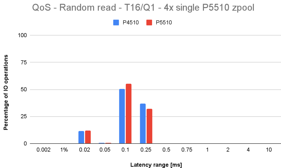
Fig. 7. Latency distribution for a random read test, done on a 4x single-disk data group zpool (T16/Q1).
