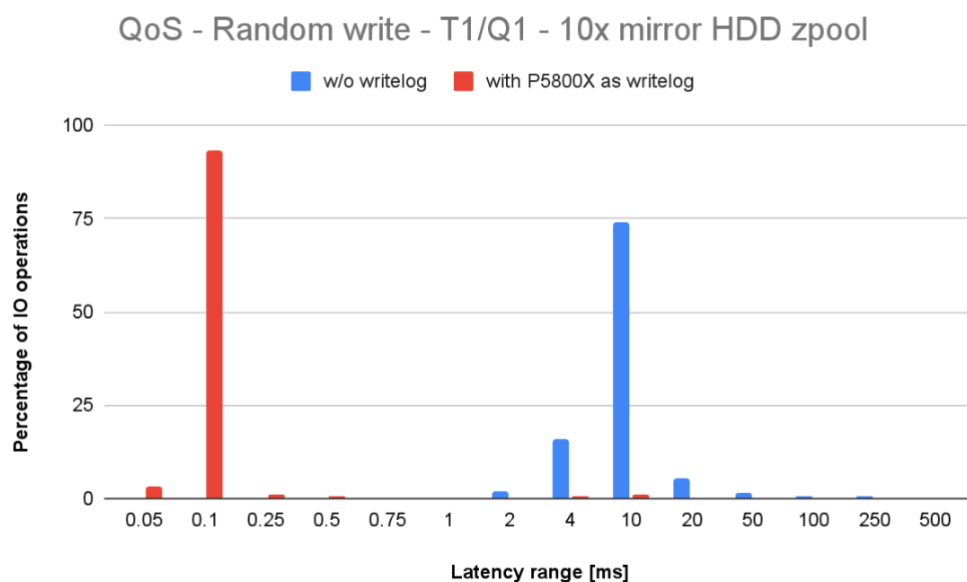
Fig. 6. Latency distribution for a random write test, done on a 10x mirror HDD zpool (T1/Q1), with and without writelog.
