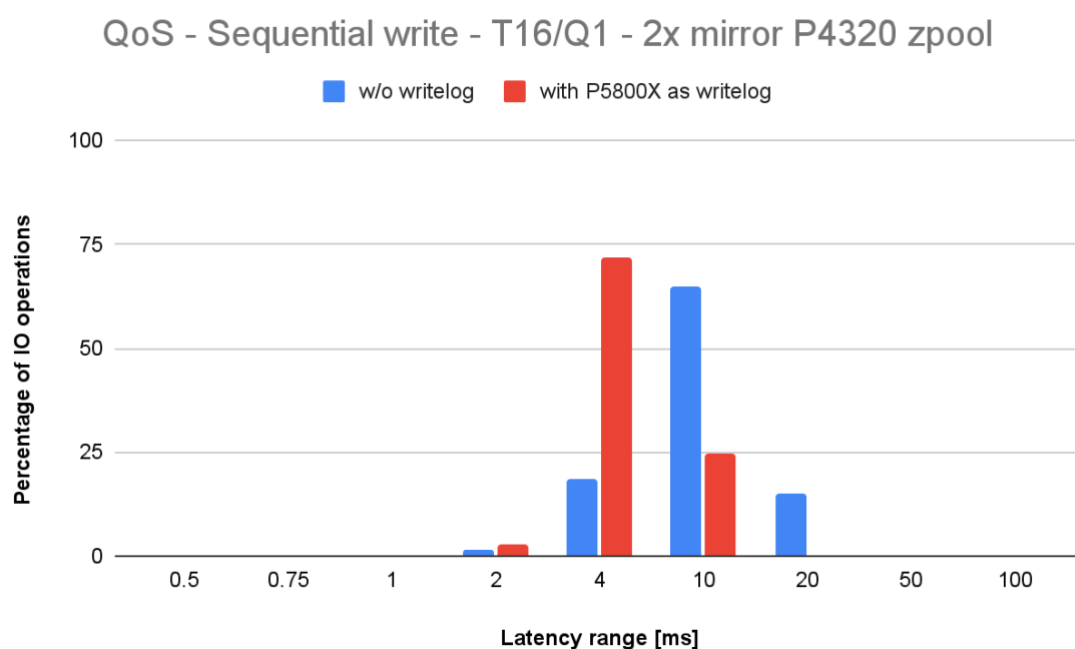
Fig. 22. Latency distribution for a sequential write test, done on a 2x 2-way mirror SSD zpool (T16/Q1), with and without writelog.
