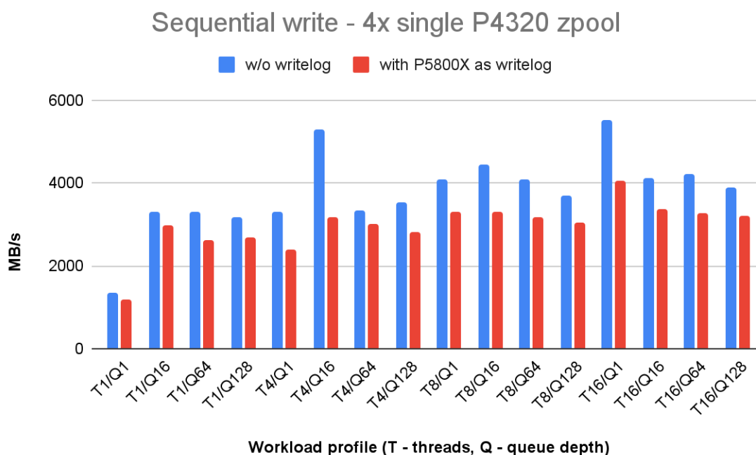
Fig. 26. Sequential write performance of a 4x single SSD zpool, with and w/o writelog.
