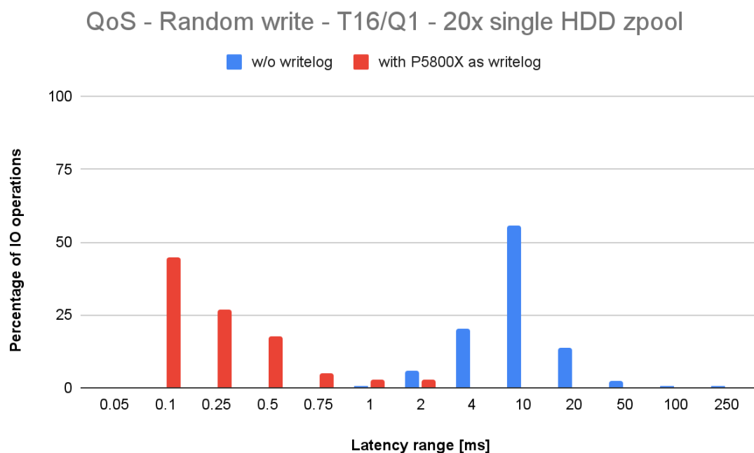
Fig. 13. Latency distribution for a random write test, done on a 20x single HDD zpool (T16/Q1), with and without writelog.
