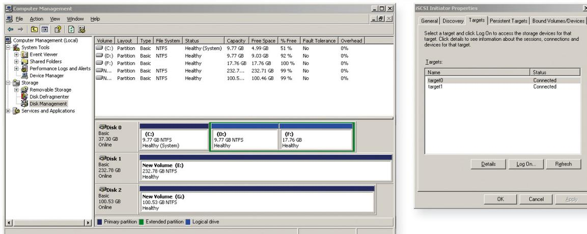
A striking advantage: Within an operating system - here Windows XP - iSCSI displays storage space on the network as a local drive, and also allows it to be managed like one.
