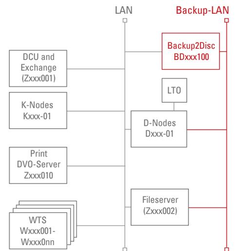
The new approach to back-up: Soon all of the field offices will be connected to the central computing center by way of a backup LAN, thereby giving them a high-performance means of backing up their data.
