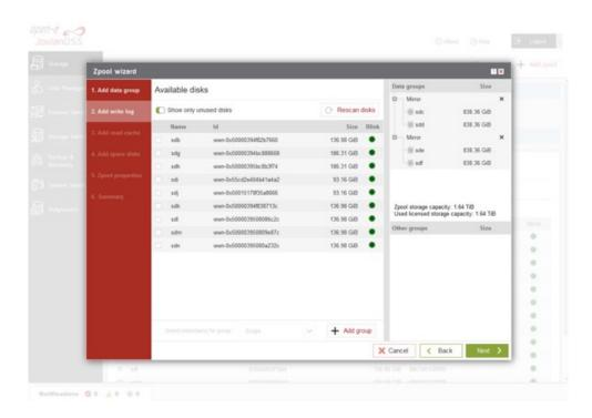
• Select the fastest disks from the list on the left and create a mirror set for the redundancy level, then click the "Add group", and then the "Next" button.
