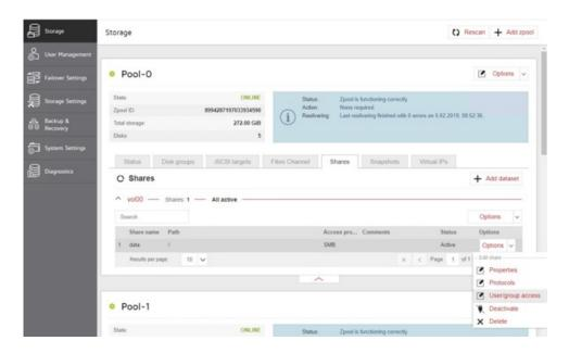
· In "Options" drop-down menu, select "Users/group access", and in "User access" uncheck the check the box with "Administrator" user, and confirm by clicking the Apply button.
