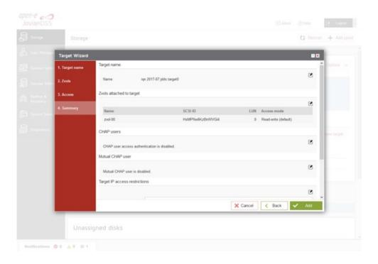
• After completion of the "Target wizard" return to the "Storage". Below you will see the "iSCSI targets" you are able to see and overview of the configuration targets.
