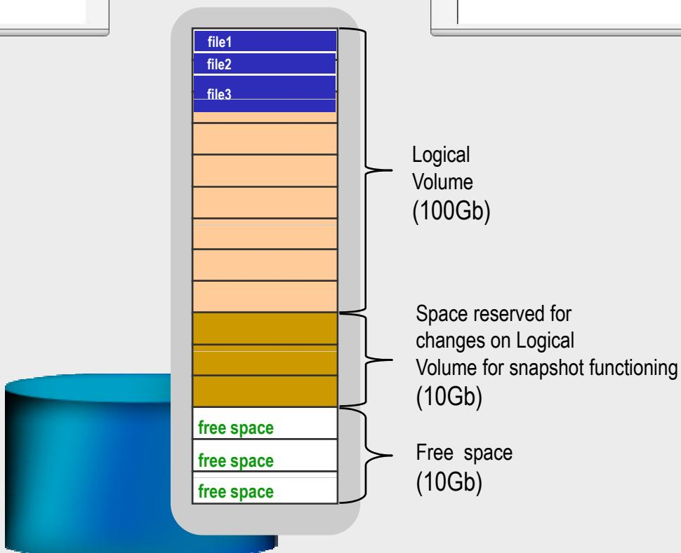
After the snapshot starts, the file system will read the data as usual, but writes will first copy the original data into the snapshot reserved space (copy-on-write) and then write new data.
