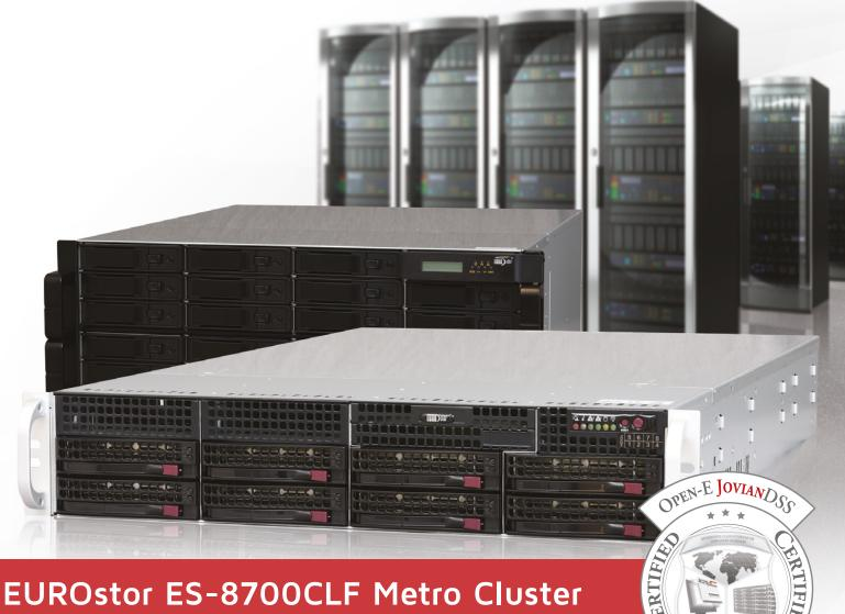
EUROstor's ES-8700CLF is an Open-E JovianDSS-based Storage Cluster for iSCSI and NAS (CIFS, NFS) access that can be set up at Fibre Channel distance. Each side consists of one cluster node and one FC JBOD connected to both cluster nodes. The disks in the JBODs are mirrored across the two locations in order to provide full site redundancy.
