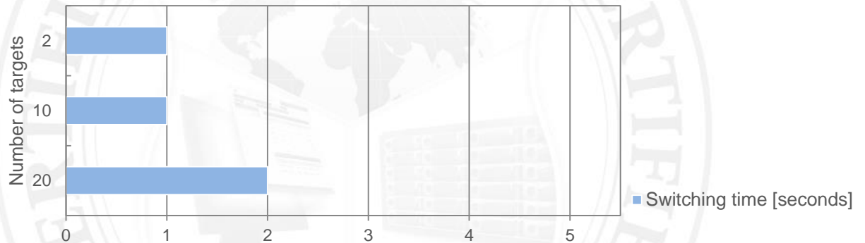
FIGURE 5: Active-Active iSCSI Failover resource groups switching time test chart for Intel® Ethernet Converged Network Adapter X540-T2 on both active nodes
