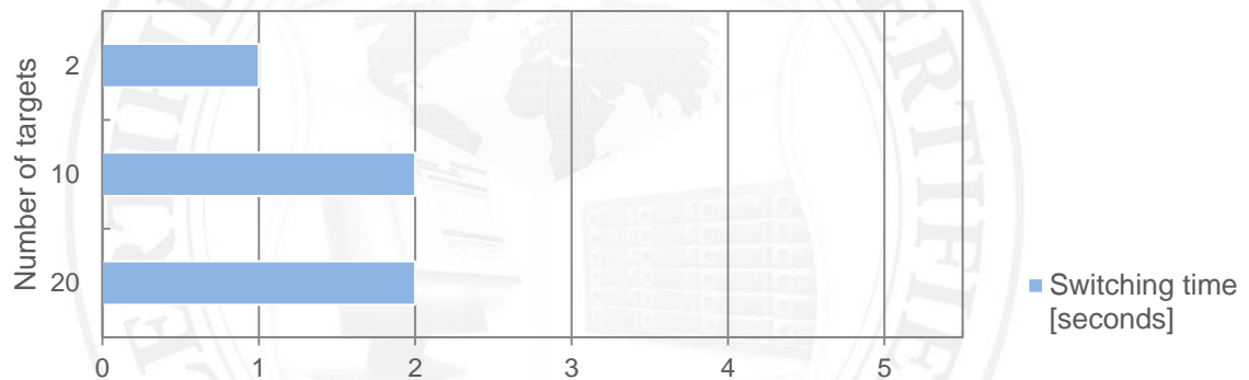
FIGURE 4: Active-Passive iSCSI Failover resource group switching time test chart for 10GbE Intel Ethernet Converged Network Adapter X520-SR2 on one active node
