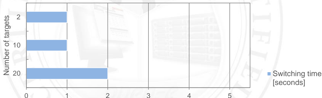
FIGURE 5: Active-Active iSCSI Failover resource groups switching time test chart for 10GbE Intel Ethernet Converged Network Adapter X520-SR2 on both active nodes
