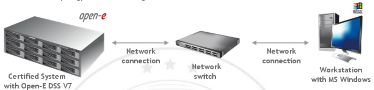
FIGURE 13: Network test topology for RAID testing
