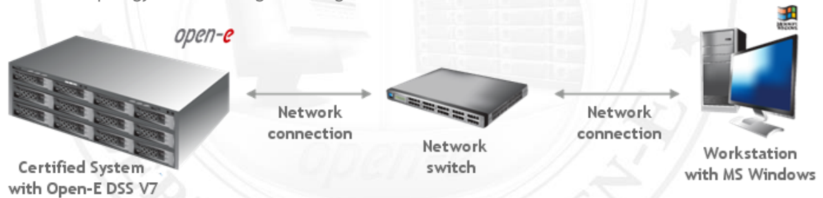
FIGURE 19: Network topology for iSCSI Target testing
