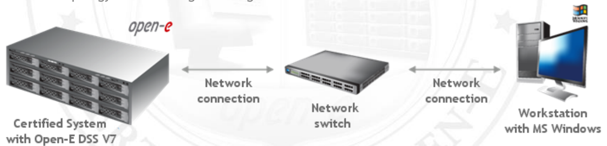
FIGURE 22: Network topology for iSCSI Target testing
