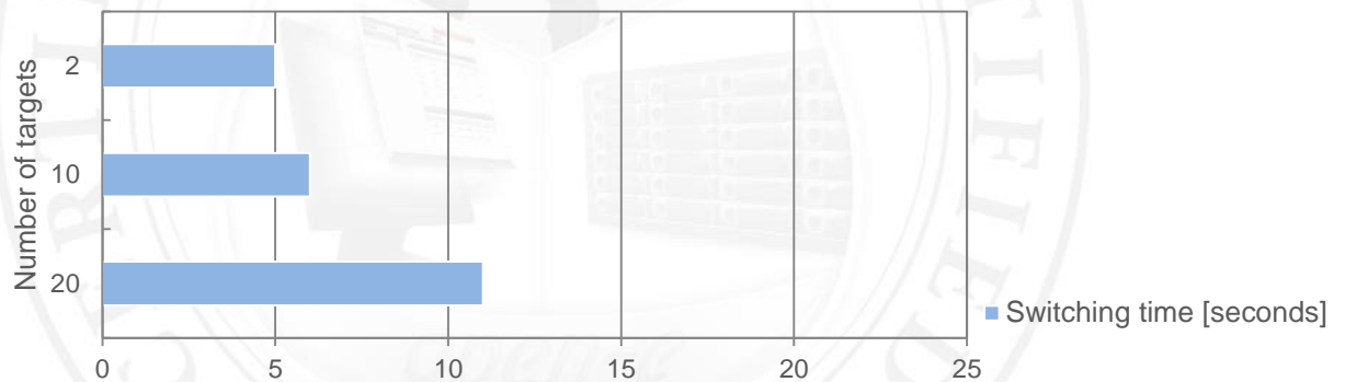
FIGURE 5: Active-Active iSCSI Failover resource groups switching time test chart for Emulex OCe14102-NT Ethernet Network Adapter on both active nodes
