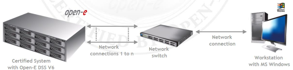
FIGURE 18: Network topology for iSCSI Target testing
