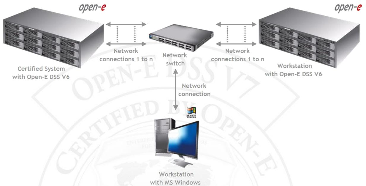
FIGURE 17: Network topology for iSCSI Initiator testing
