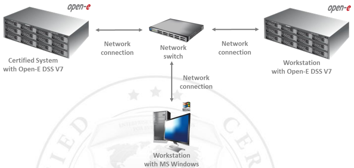
FIGURE 19: Network topology for iSCSI Initiator testing
