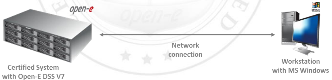
FIGURE 20: Network topology for iSCSI Target testing
