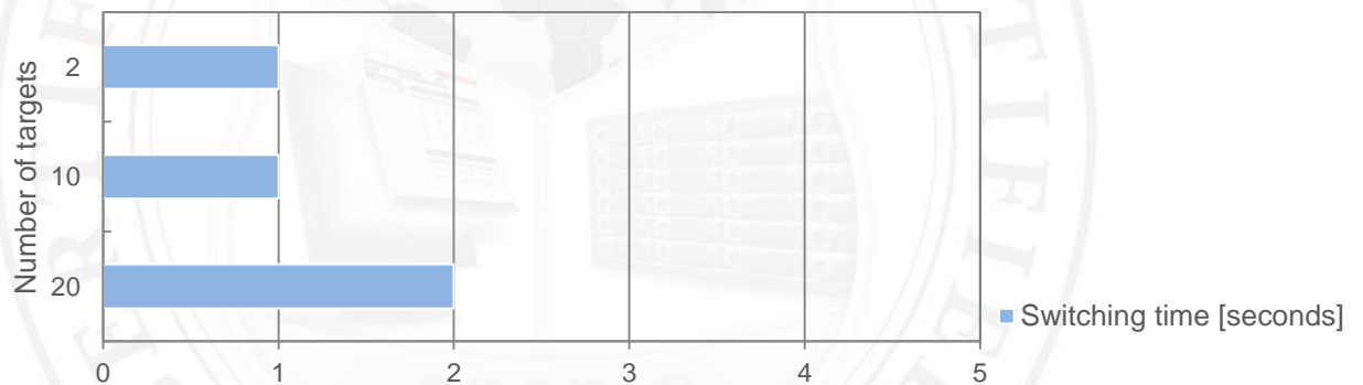
FIGURE 5: Active-Active iSCSI Failover resource groups switching time test chart for QLogic QLE3442-CU (Dual Port 10GbE) with MPIO
